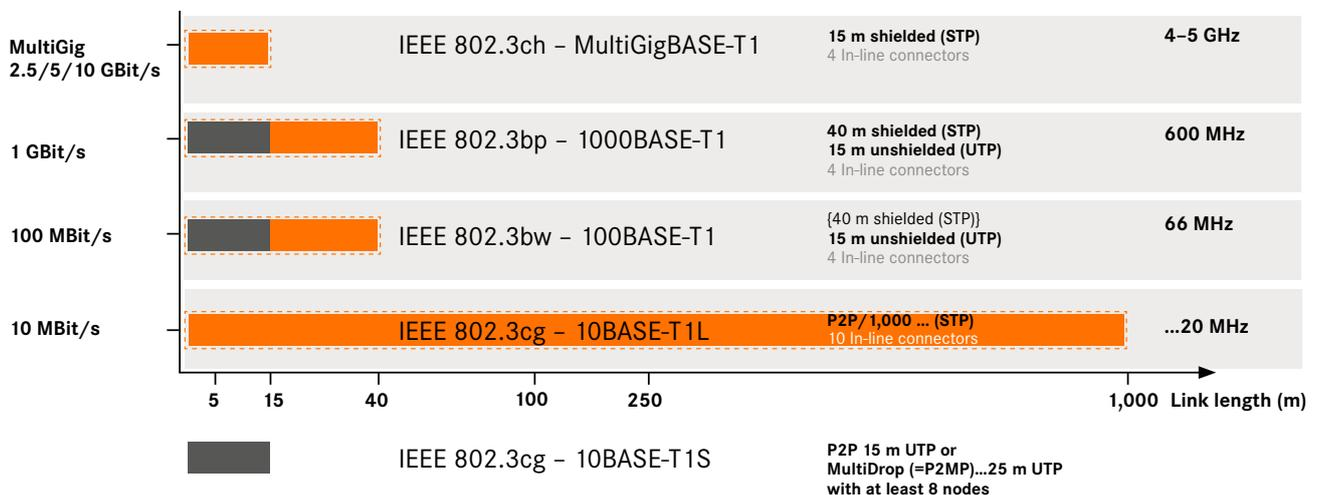
Figure: Overview of the IEEE protocol standards for Single Pair Ethernet
